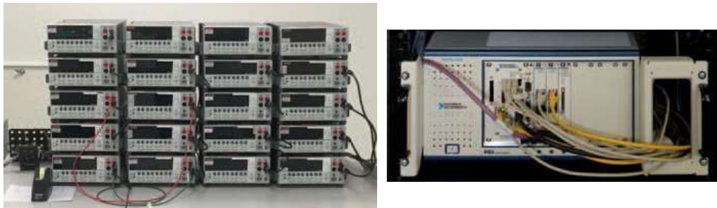
Figure 14.30 A PXI-based data acquisition system compared to a stack of conventional instruments.
