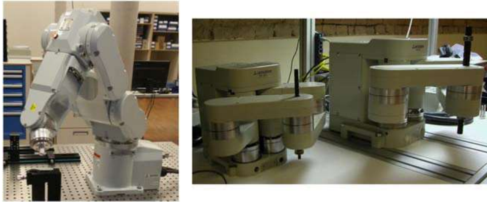
Figure 14.14 A 6 axis EPSON C3 and two Mitsubishi parallel robots (see text).
