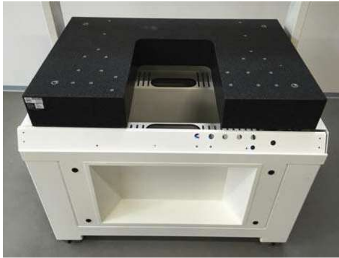
Figure 14.16 A hefty granite optical table mounted in an enclosure with isolation support pads.
