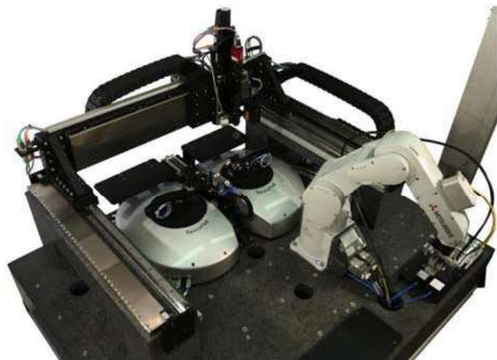
Figure 14.7 A pre-production PICs assembly machine designed and built in 2013. Source: Courtesy of PI-miCos.
